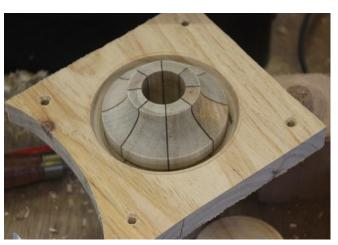
faceplate and try it on the budvase. It should be a firm fit and cover the groove. Replace the square wood onto the faceplate and enlarge the hole to half of the depth. Make the hole about 8mm diameter bigger than it was and taper the cut. Now replace the square piece of wood on the
