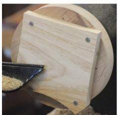
Now screw a piece of scrap timber about 160mm square and 19mm thick onto a wooden faceplate. Mark its position so that the wood can be put back if required. Bring up the tailstock to bear against the wood. Now use callipers to measure the diameter of the turning near
