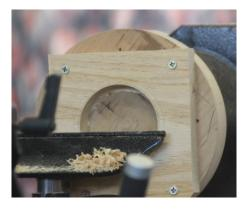
the groove. Mark this dimension on the square piece of wood. Make a deep groove between the marked circle and the centre, deep enough that the centre piece becomes detached from the
