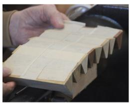
The staves should be placed side by side with the 45degree angle down and the 30mm face uppermost. One strip of masking tape is then placed to connect the pieces. After turning them over, the staves can be rolled up to make a circular form about 80mm diameter. If the 45-degree angle is accurately formed, the end pieces will meet with no gaps. If that has been achieved, then the staves can be opened out and more masking tape applied.
