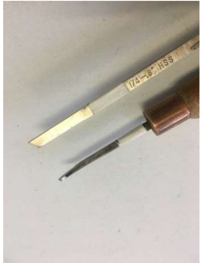
(Right) Scraper and hollowing tool made from and Allen Key
