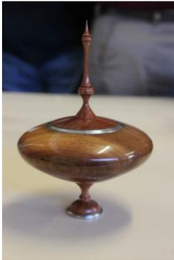
Frank Larsen's Cindy Drozda inspired lidded container uses Blackwood, Jarrah and pewter. He has also made another with an ebonised finial. The decorative pewter rings are rough-cast in timber moulds from melted-down op shop pewter mugs and dishes, then finished by turning with standard gouges.
