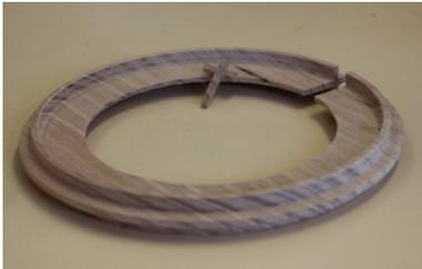
This is an example of something "square" which was turned on a lathe. The little Mountain Ash crosses for earrings are cut out as the cross-section of a large flat ring which has a raised thin "spigot" on each side. Very precise turning required in order for the sections to look crisp
