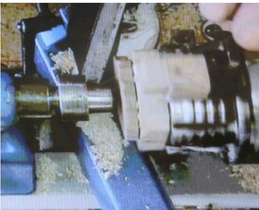
Until the blank broke, Val started to show us how he shapes pendants, using a chuck jig to control the workpiece offset. He attaches a thin blank with double-sided carpet tape, and uses the tailstock for security while turning the face and edge, then removes the tailstock to finish the centre, and sand the face and edges. He then loosens the screws on the jig to move the turning centre, in order to cut a decorative groove and drill the hole for the neck cord.
