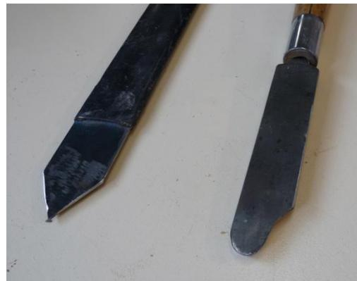
**Home made tools;** Special profile tool to turn bell shaped ends. Parting tool is made from old industrial hacksaw blade. Ring & cone drive spur turned on lathe, metal softened by heating and slow cooling.
