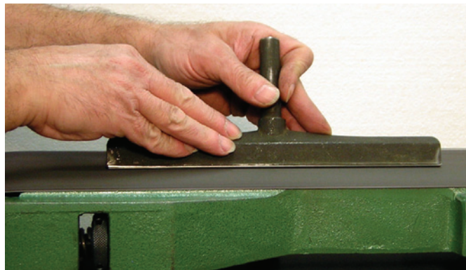
Photo 5—Smooth the top surface and remove all sharp edges from the tool rest with a belt machine as shown, or with a file.
