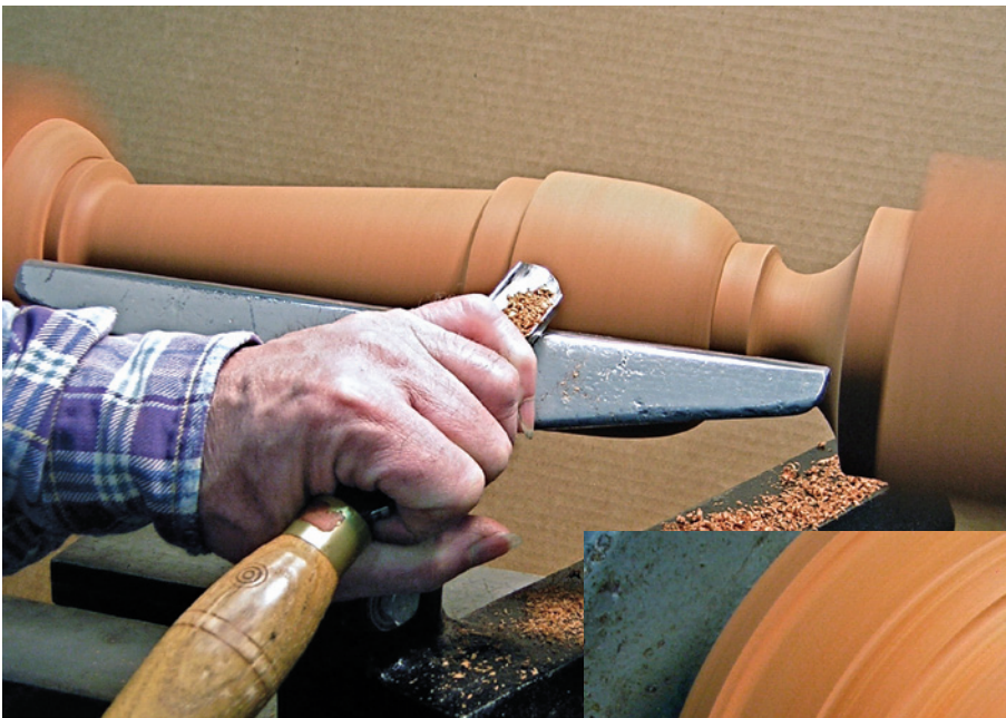
Photo 8—For spindle turning, and often on the outside of a bowl, the tool rest is placed above center. It should be possible to raise the tool rest at least \frac{3}{4} " above center.
