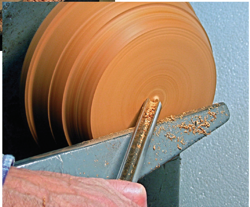
Photo 9—To reach the center of a face turning, the tool rest must be below center. It should be possible to lower the tool rest at least \frac{3}{4} " below center.
