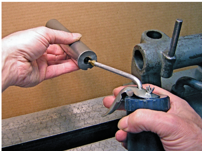
Photo 4—Remove the ram completely, check for damage to the surface, lubricate the threaded hole and the outside surface before reassembly. On small lathes, the ram is threaded externally and has no central screw.
