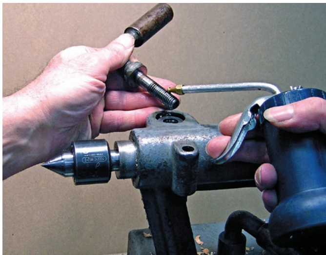
Photos 2 & 3—Remove the screws completely, clean them, and oil generously before reassembly.
