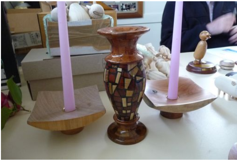
Blackwood Candle stick holders and Vase by Ron Dunstan. Vase is constructed of 331 pieces of wood. Joints filled with timbermate. Polyurethane finish. Great way to use up those leftovers.
