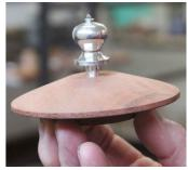
Charles uses scrapers and parting tools to shape pewter, and has ground a semi-circular end on an old wood chisel for this purpose. He polishes the pewter with 400-1200 sanding pads, and finally with car polish.
