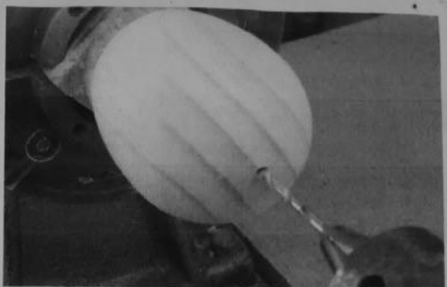
Photo.4: Drilling the hair blank to take the dowel for the bow
