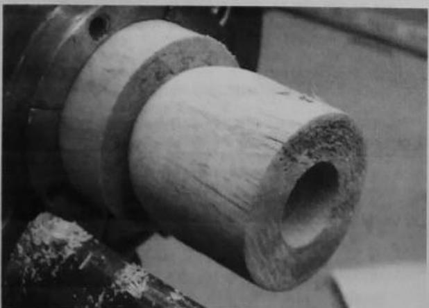
Photo.8: Drilling the head for the connecting dowel and shaping the lower curve of the face
