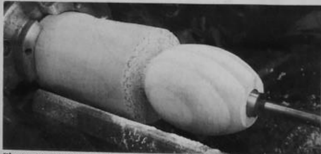
Photo.10: Drilling the body for the connecting dowel
