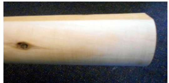
Crisp edge obtained by using sanding block on non-round item
