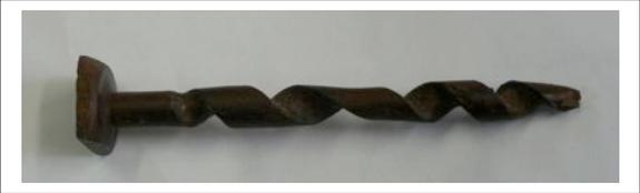
To make this 'screw ribbon' David uses a micro plane and rasp held at about 45 degrees to remove wood at the same time turning the lathe very slowly by hand.
