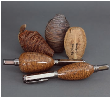
Very papery on the outside and ready to crumble at a moment's notice, the Deodar Cedar cone ( Cedrus deodara ) does have some woody material in it, but the lack of structural integrity requires CA glue to be applied early on. The pattern made by the stabilized paper scales is lovely.
