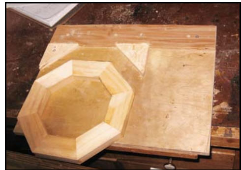
Figure 5. Octagonal Ring and Bench Hook-Plane Stop. The triangles are just screwed to the bench hook. The right-hand one is easily adjustable for various sized rings.
