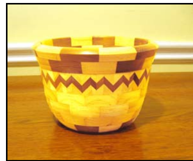
Figure 17. Segmented Bowl with Zig-Zag Feature Ring. Note irregularities in the zig-zag design
