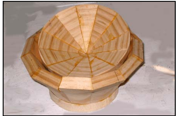
Figure 14. Two Staved Bowl Blanks. Note that the raw ends of the staves are sharp arrises, unsuitable for gluing. The bottom of the larger blank has been planed off on a lathe to make a flat surface for attaching the bottom disc.
