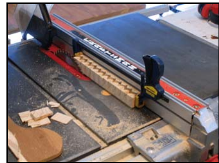
Figure 16. Trimming the Zig-Zag Pieces (The pieces are resting on a Masonite sled, held in place by double-sided tape.)
