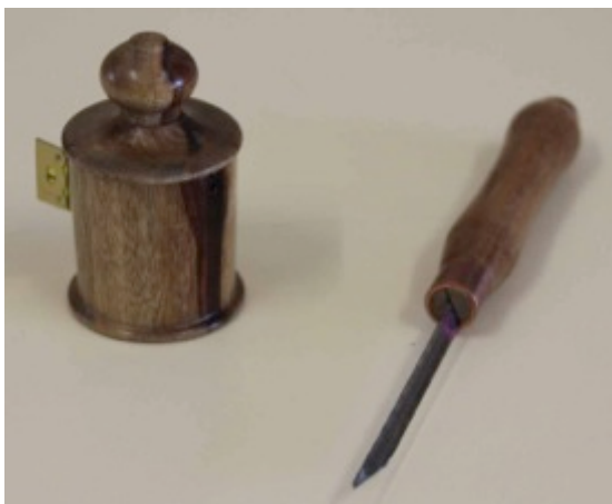
Alan Thompson brought his Camphor Laurel tape measure from last month, and the improvised tool for cutting a narrow slot – a ground-down hacksaw blade with handle.
