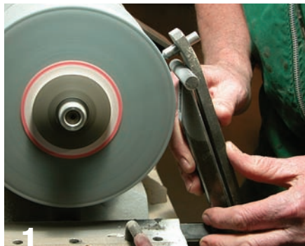
1 Regular use of a wheel dresser will true your wheel and expose fresh grinding surfaces.
