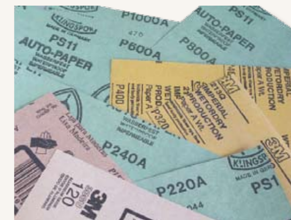
BELOW: Proper preparation for applying a finish requires working through all of the grits. Slow speed to build minimal heat and allow cutting, including cleaning between grits yields quality results
