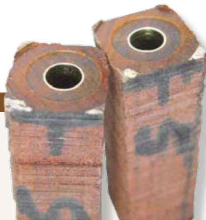
ABOVE: Facing the blanks should expose the tube just flush with the blank. Piloting on the inner diameter of the tube will provide the most perpendicular surface during the facing process
