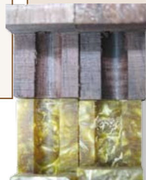
BELOW: Proper drilling technique will yield quality size and surface for the adhesive bond. Excessive force or speed will melt and cause dimensional variation or polish the inside of the hole reducing adhesion
