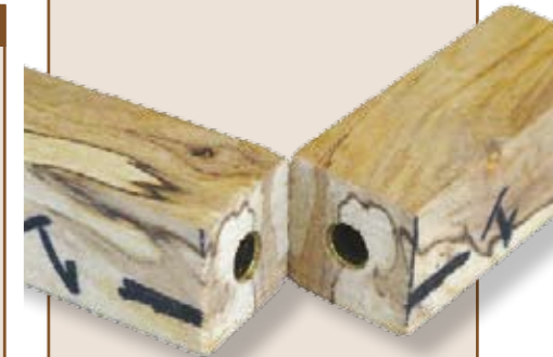
ABOVE: Use the matching cut ends when gluing in your brass tubes. To preserve grain match, keep the tubes as close to the surface as possible allowing for proper facing with minimal material removal
