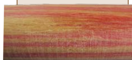
ABOVE: Use both radial and axial sanding to achieve the best results. The axial sanding on the top portion of the blank with the same grit shows how it can 'erase' the original radial scratches
