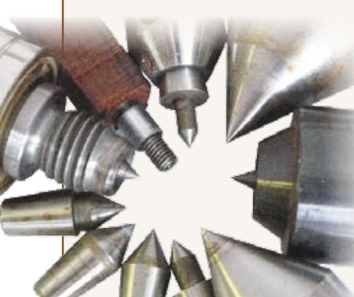
LEFT: The points on tailcentres vary in tip angle. This potential mismatch with the mandrel end encourages the user to use excessive force on the tailcentre to compensate
