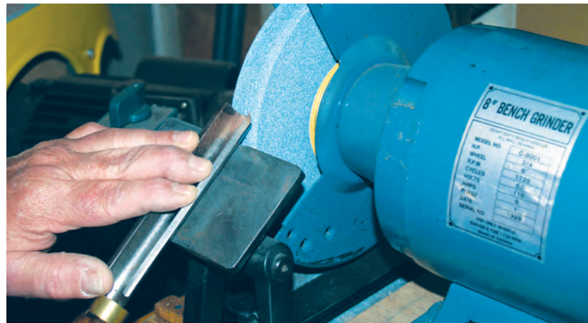
Consider learning how to hand sharpen turning tools. This allows you to place a toolrest close to the grinding wheel, eliminating many potential dangers.
