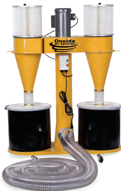
Oneida Air System's portable collector is designed for woodworkers and turners who don't have a central dust collection system with lots of ductwork already in place. The cyclones create a vortex that uses centrifugal force to separate dust from chips.
