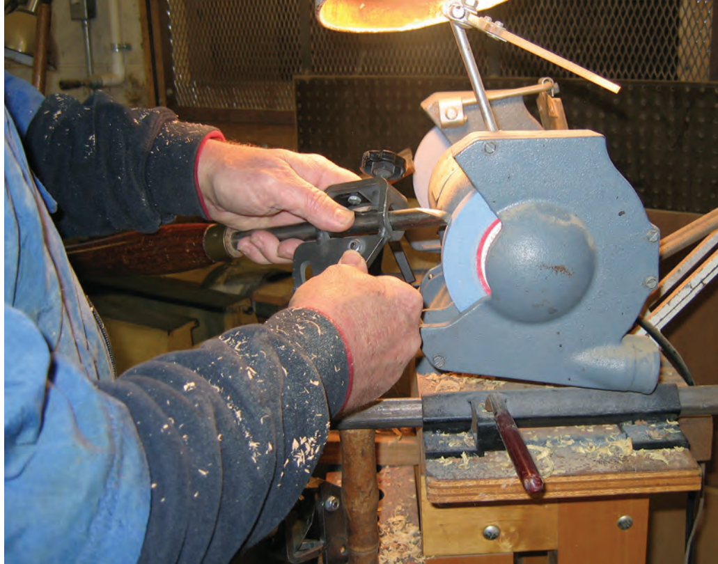
A grinding jig helps many new turners repeat the same bevel on a lathe tool.
