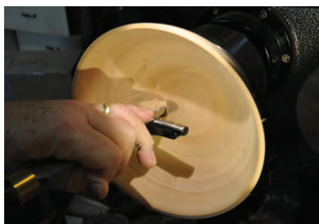
When using a scraper on the inside of a bowl, make sure the toolrest is as close as possible to the surface being cut. You might even want to use a curved toolrest. Use plenty of light.
