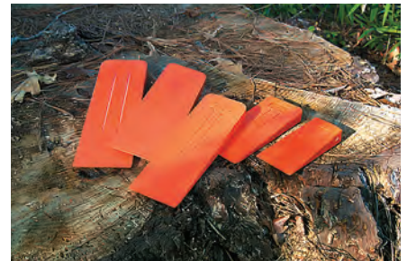
Use a polymer wedge (available from a chainsaw store) to keep the kerf open in deep cuts. If you accidentally knick the polymer wedge, you won't damage the chain.
