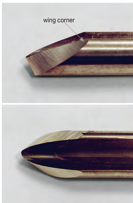
The wing (side) profile of Lyle Jamieson's favorite grind has a nearly straight line from the tip to the wing corner.
