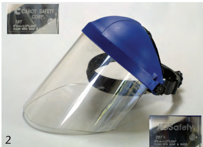
This faceshield has a thick polycarbonete shield. Note the impact rating in the inset images, basic impact, Z87 (upper left) and high impact, Z87+ (lower right).
