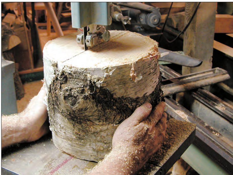
With 6"-diameter or larger stock, you can bandsaw logs upright to halve the material. Note safe hand position.
