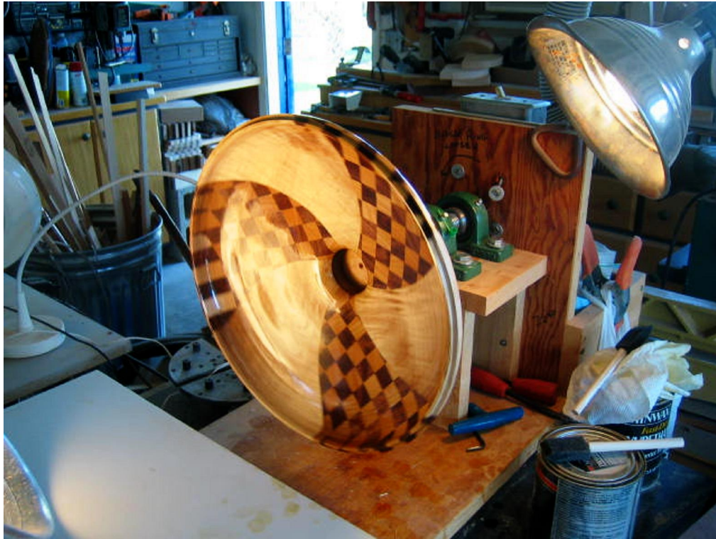
I have finished turned and sanded both halves and finishing on my Slow Turn Finsher.
