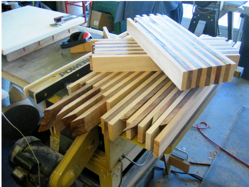
Glue up stock for 3" thick Checkered Blanks 11 strips @3/4"
