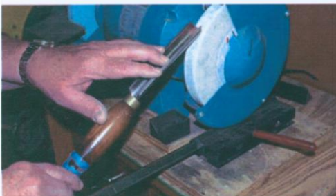
Better: Create a more acute bevel angle on your tool, which will place it higher up on the wheel in a safer position
