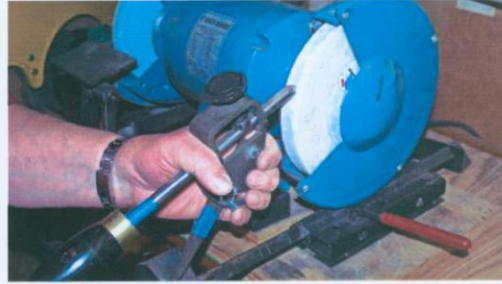
Wrong way! If the sharpening jig slips, fingers will contact the
