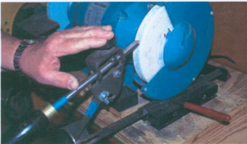
A safer way to hold the jig is on the top. If a slip occurs, the hand is protected.
