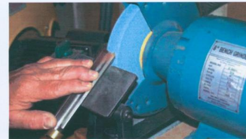
Consider learning how to hand sharpen turning tools. This allows you to place a toolrest close to the grinding wheel, eliminating
