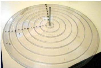
Peter starts by preparing a suitable blank of close grained timber such as Red Gum, Leatherwood or Myrtle (in this case a 300mm by 40mm piece of Tas Myrtle). He uses the jig at left to mark the circle and uses the nail to mark centre prior to cutting out on the bandsaw.
