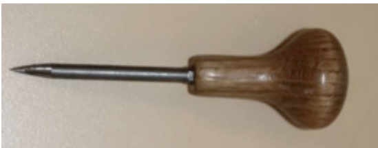
Richard Jardine made the awl handle from Tallow Wood, finished with Glow. The tang is a sharpened hexagonal screwdriver blade.
