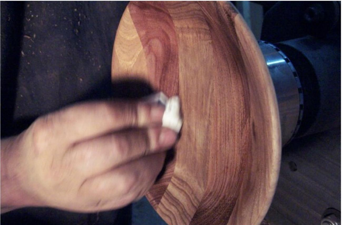
Again, step aside and start lathe. Work the shellwax from the centre in a slow even movement
