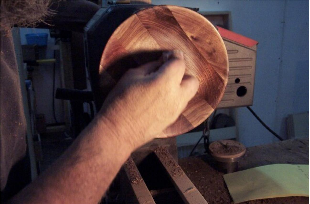
Once you have the EEE on, step aside (saves excess splash on you ) and start the lathe. The revs should be as fast as the article will go safely. This was turning at 2000 RPM.
