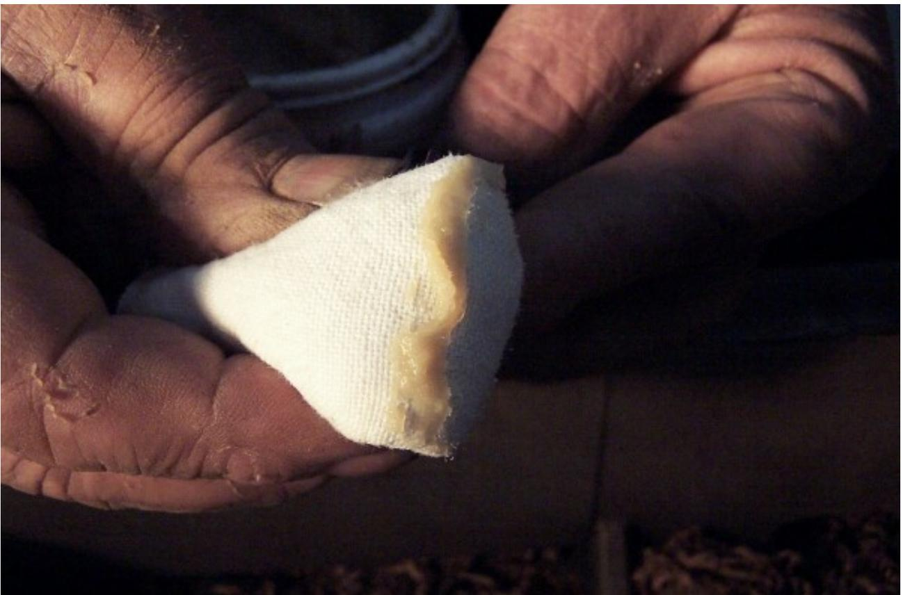
With the lathe stopped, quickly wipe the contents lightly over the bowls surface. This requires a
